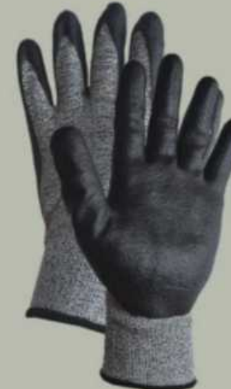
ITEM NO:DM6087 Description: 13 gauge HPPE+glass fiber mixed liner with nitrile foam coated on palm cutting gloves Anti-cut Level:3/5
