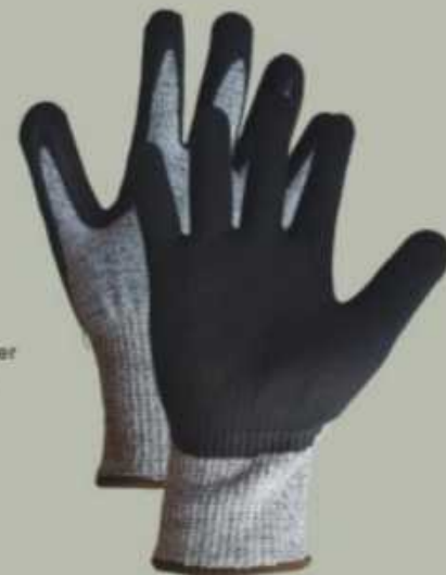
ITEM NO:DM6086 Description: 13 gauge HPPE+glass fiber mixed liner with Latex foam coated on palm cutting gloves Anti-cut Level:3/5
